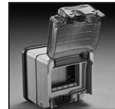
684638X45 Weatherproof Cover & Box. Gray. IP66. Surface Mount. Accepts 22.5mm, 45mm & 67.5mmx45mm Devices.
